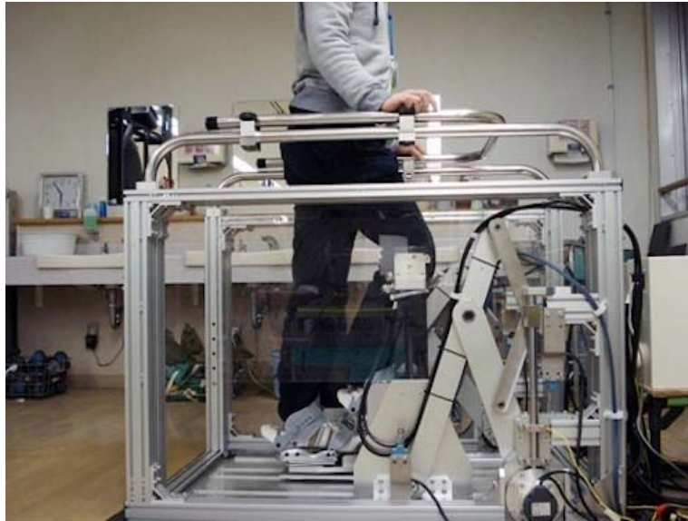
20 example. GaitMaster 5 simulator created Tsukuba University researchers in Japan
